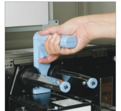
Vertical lifting head unit for easy access
